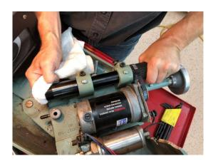
Insert collet and thread the nut onto the spindle.
