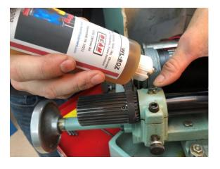
with grinding stone debris, metal chips, or any other such debris will irreversibly damage the spindle). Also, refrain from using excessive or blunt force on any part of the Tru-Valve spindle assembly. When dressing the valve facing stone with the diamond dresser it is best to cover the collet so that no stone dust gets into the collet.
