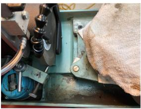
The Tru-Valve Spindle assemblies and the collets are precision pieces and should treated as such by being kept clean and free from any debris (tightening a collet in the spindle housing
