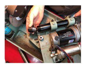
Insert your valve into the collet to your desired depth and tighten the nut. (The nut only needs to be snug or hand tight in most cases. In other words, use the wrench to just hold the nut with
