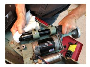
Insert collet and thread the nut onto the spindle.
