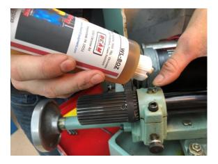
The Tru-Valve Spindle assemblies and the collets are precision pieces and should treated as such by being kept clean and free from any debris (tightening a collet in the spindle housing
