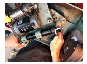
When removing do the reverse but you will need to turn the nut back far enough to pop the collet out of its seat to release the valve.
