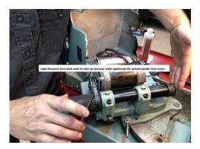
The next step is to place the belt back onto the motor pulley and end of the spindle shaft. Now take the splined handle and slide it onto the Spidle shaft and into the cog drive belt.
