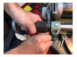
the spindle. Back them off several turns so they are completely free of tension.
